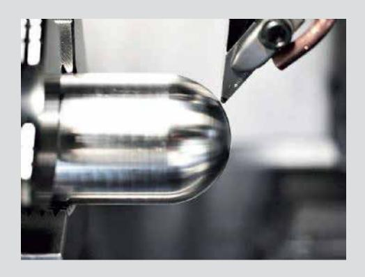
PCBN and PCD are high-performance tool material from a polycrystalline mass, produced in high temperature-pressure process.
